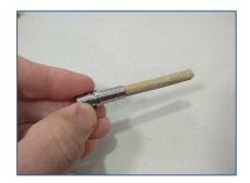
2. Clean the inside of the Connector Shell with a lint-free wipe soaked in acetone and allow to dry. If using a primer (recommended for urethane), apply the primer to the inside of the Connector Shell using a cotton swab or equivalent and allow to dry.
